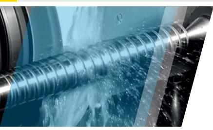
These fluids offer the highest level of cooling, best workplace visibility, and are formulated to minimize operator sensitivity. These fluids are low foaming which is ideal in high-pressure coolant systems and also offer good detergent properties for maintaining free cutting grinding wheels.
